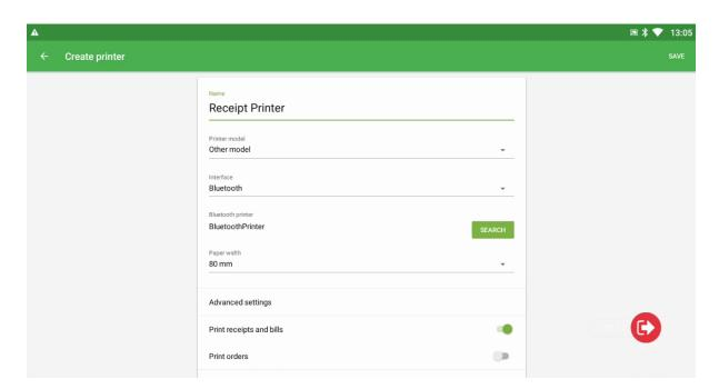
Once these options have been set, click *Advanced Settings*. Under the section that says *Initial ESC/POS commands*, you will want to set the value of *Drawer ESC/POS commands* to the following value: **10,14,00,00,00**. It will automatically input the commas, so you just need to enter the numbers. It should look the same as below:
