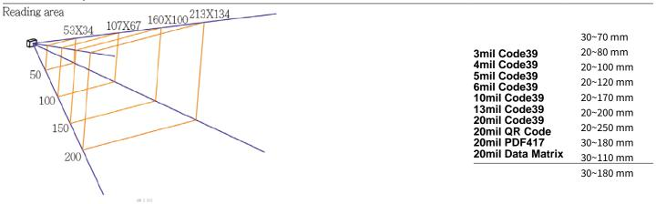
Note: the test is under ambient light 700  $\sim$  800 Lux.
