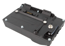
94ACC021(6/7) TaskBook Docking Station with Lever Lock
