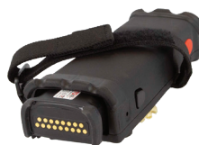
94ACC0222 Hot swappable battery for handgrip
